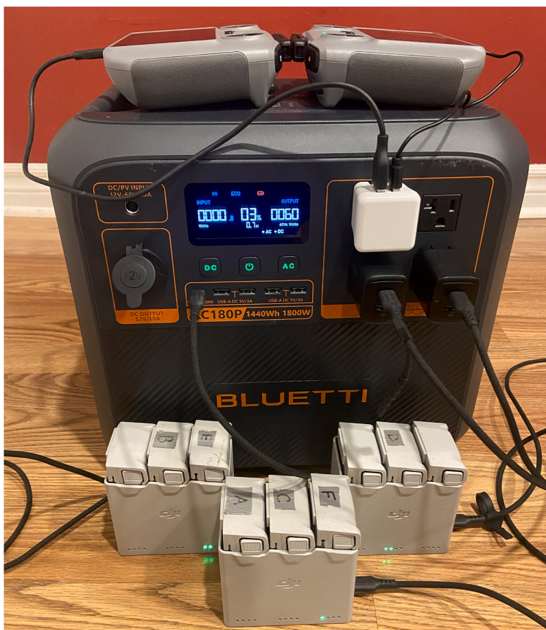
Fig. 4. Charging station used in a study of painted turtle basking behaviour at Kenauk, Montebello, Québec, Canada, in 2025. The charging station consists of a Bluetti Portable Power Station powering three individual DJI Two-Way Charging Hubs with 30 W USB-C chargers, each charging three DJI Intelligent Flight Battery Plus units, for a total of nine batteries.
