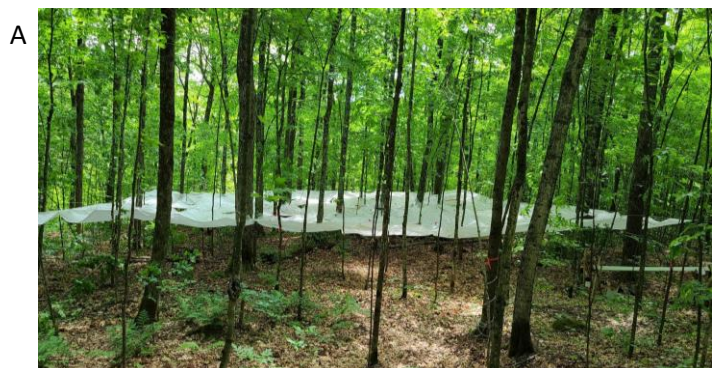
Figure 4. A) Photo of the precipitation exclusion device. B) Experimental design of sites with and without beech proliferation and with and without precipitation exclusion.
