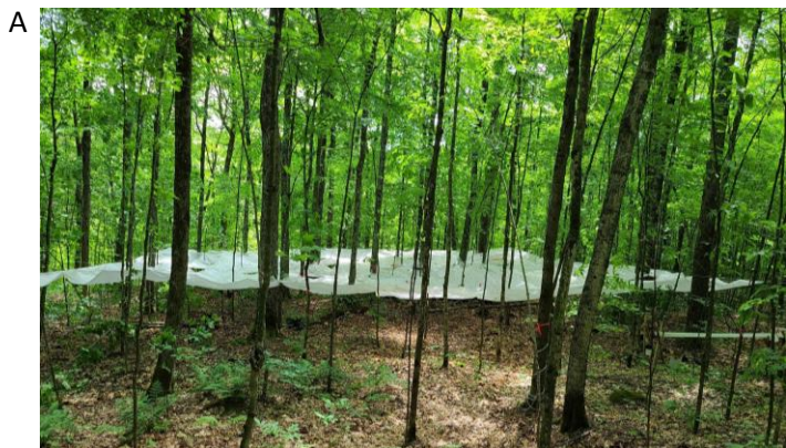
Figure 6. A) Photo of the precipitation exclusion device. B) Experimental design of sites with and without beech proliferation and with and without precipitation exclusion.
