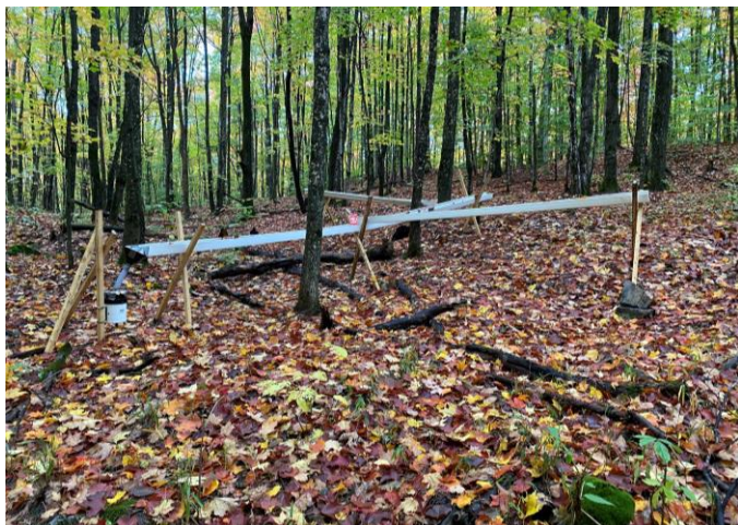
Figure 9. Monitoring precipitation interception by the forest canopy.
