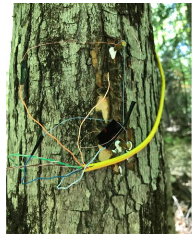
Figure 10. Monitoring tree transpiration using sensors that measure sap flow.
