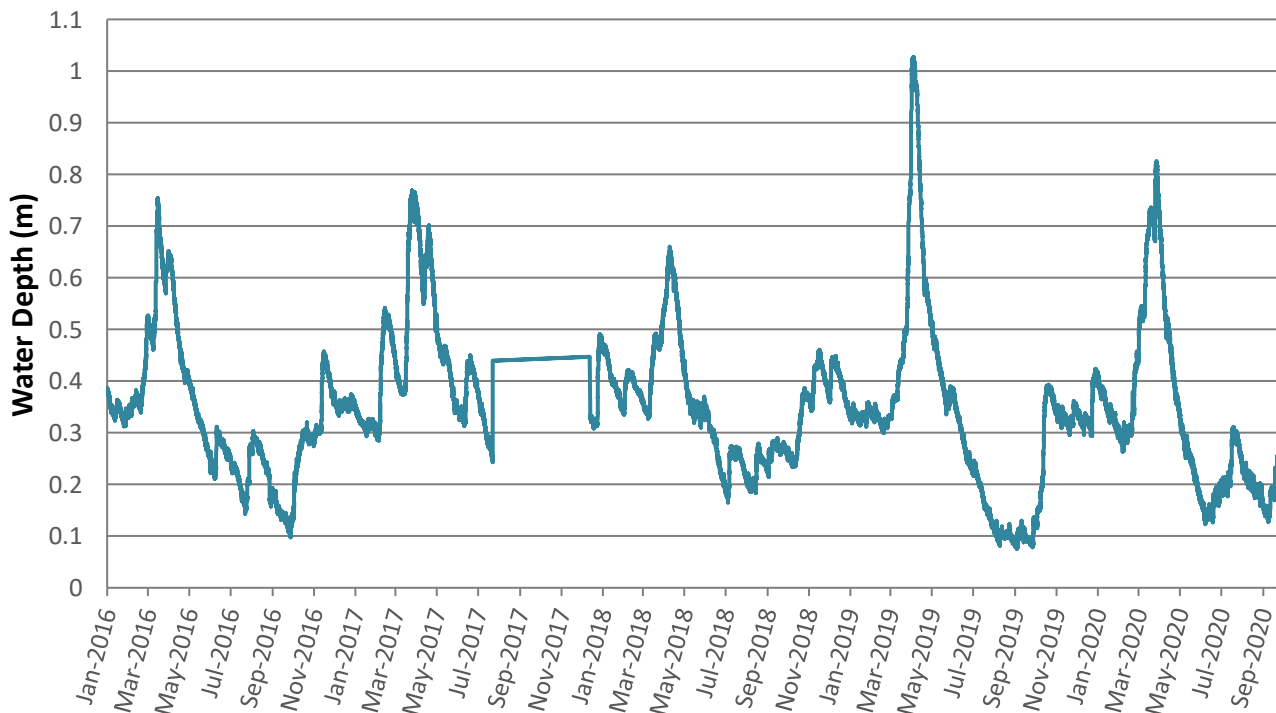
Figure 23. Water depth above the weir. *Note that water depth was compensated for barometric pressure and the data for 2020 does not include the whole year yet (data ranges from Jan 1 to Oct 16, 2020).
